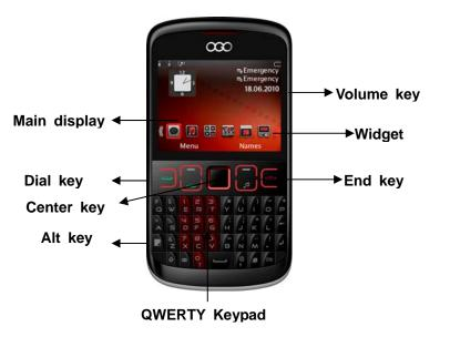
Home key (optical mouse); Simulate the navigation keys, used it to highlight menu. Move the cursor location and so on.
